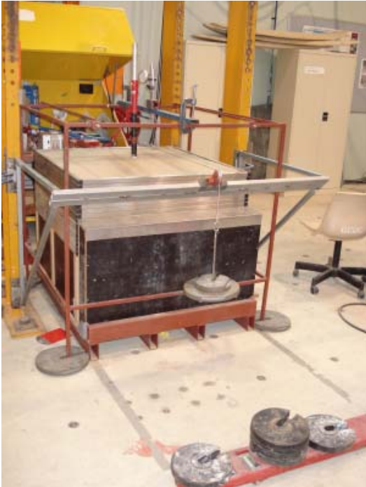
Figure 2-5: Test setup with lateral load applied.
