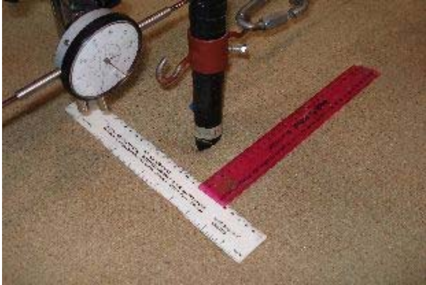
Figure 3-9: Measuring of hole behind pile.
