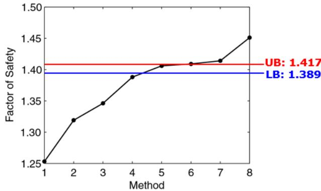
Figure 2-3: Comparison between limit equilibrium and limit analysis for slope stability.
