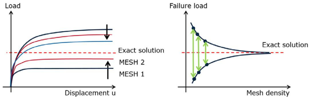
Figure 6-1: Design process for FELA, courtesy of OptumCE
