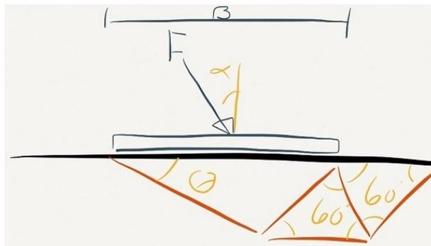
Figure 3-2: Kinematically admissible solution
