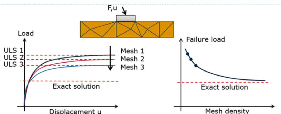
Figure 5-1: Design process for FEA, courtesy of OptumCE
