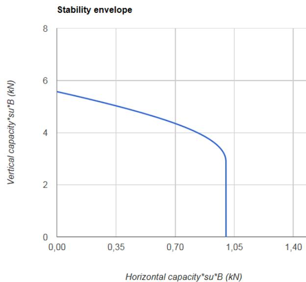
Figure 3-3: Stability envelope based on a kinematically admissible solution
