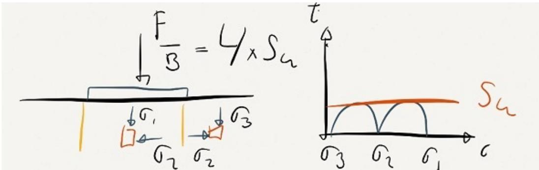
Figure 3-1: Static admissible solution
